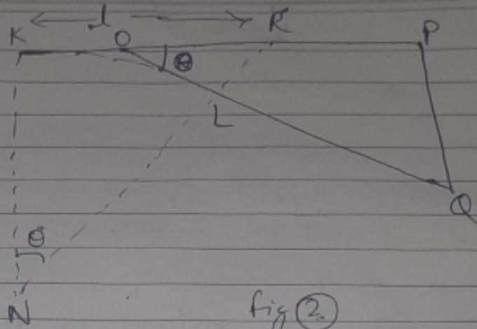
undeflected spot and  $Q$  is the position of spot deflected in the presence of magnetic field alone. The electron ~~travels~~ traverses circular arc  $KL$  centred at  $N$  in the magnetic field.
